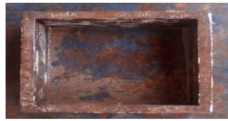
Plate 1. One of the 15 fabricated molds with 65mm by 55mm and 25mm-depth cavities for coating the plates
