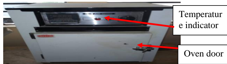
Plate 3. Front view of the oven used for heat-maintaining bitumen samples at 150^{\circ}\text{C} \pm 2 in steel containers
