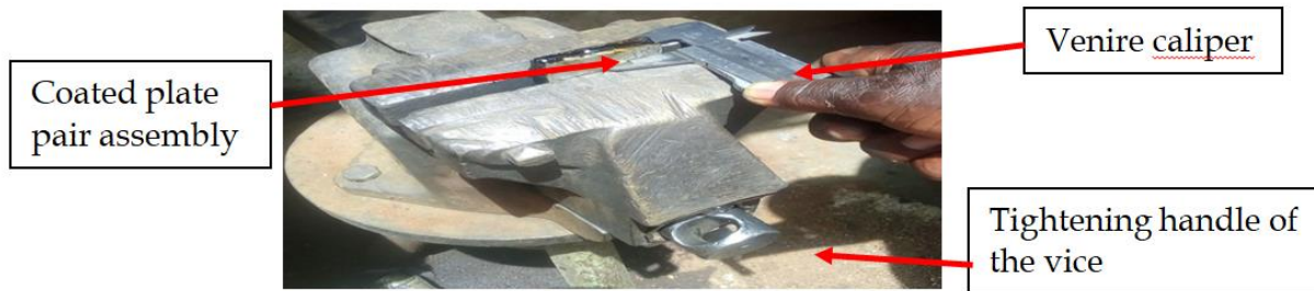
Plate 4. An instance of compressing plate pair assembly to achieve requisite coating thickness with a precision vice jaws and a micrometer
