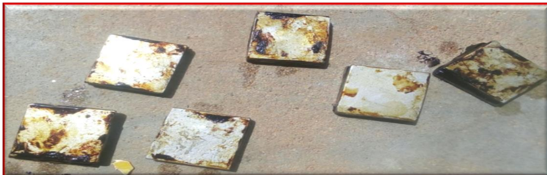
Plate 5. Some plate pair assemblies with 0.81mm-thick coating achieved between them
