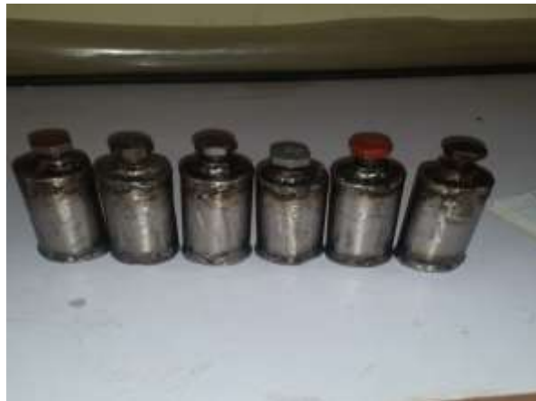
Fig. 2: Stainless steel capsule completely fabricated
