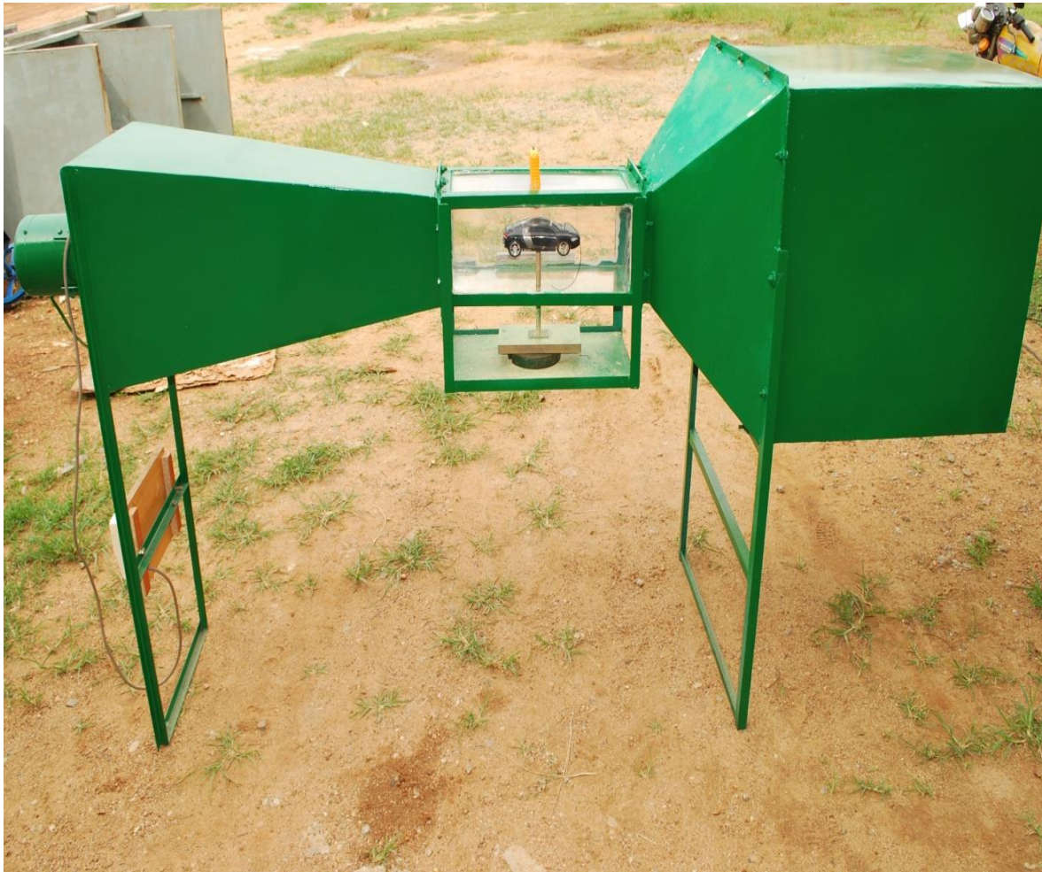
Plate 1. Fabricated low-speed open circuit wind tunnel
