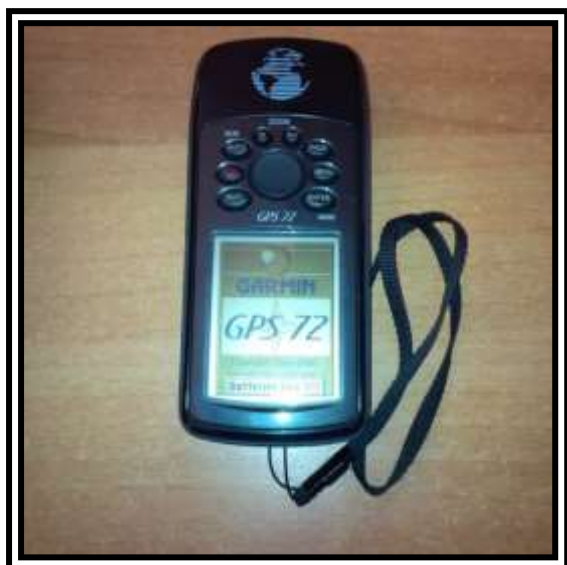
Fig.1 Garmin GPS 72 receiver used for geo-location of sampling points
