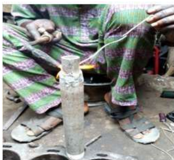
(a) Joining of the mixer chamber to the throat section
