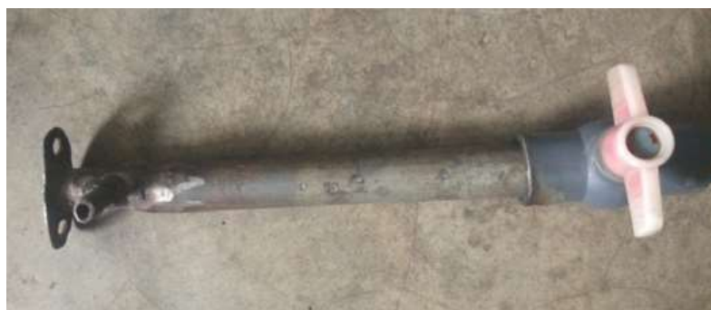
Fig. 3 The venturi mixer
