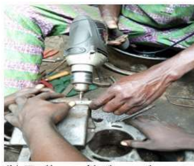
(b) Drilling of holes at the orifice section
