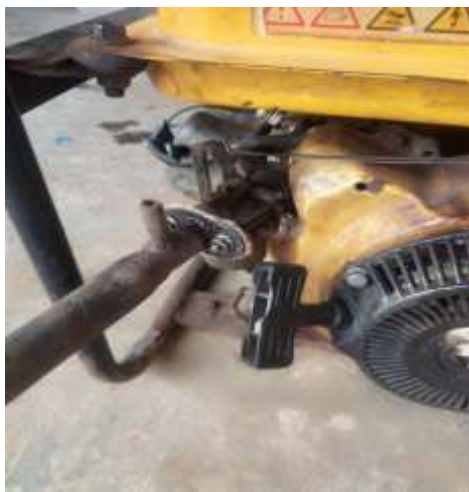
Fig. 4 Mounting of the venturi - mixer to engine
