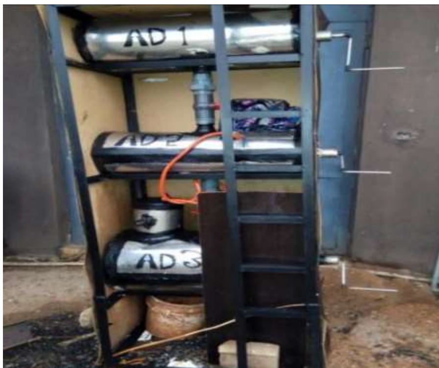
Fig. 3 Fabricated three-stage continuous anaerobic digestion plant
