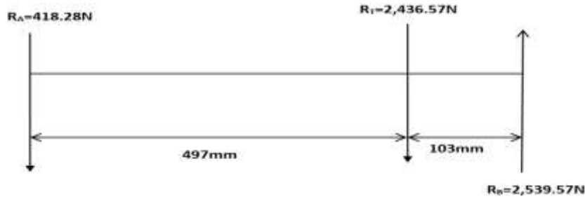
Fig. 3 Shearing force diagram analysis
