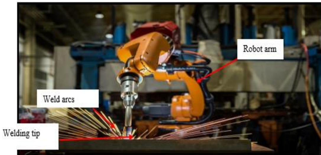
Fig. 1. An instance of robotic welding (ATI, 2021)
