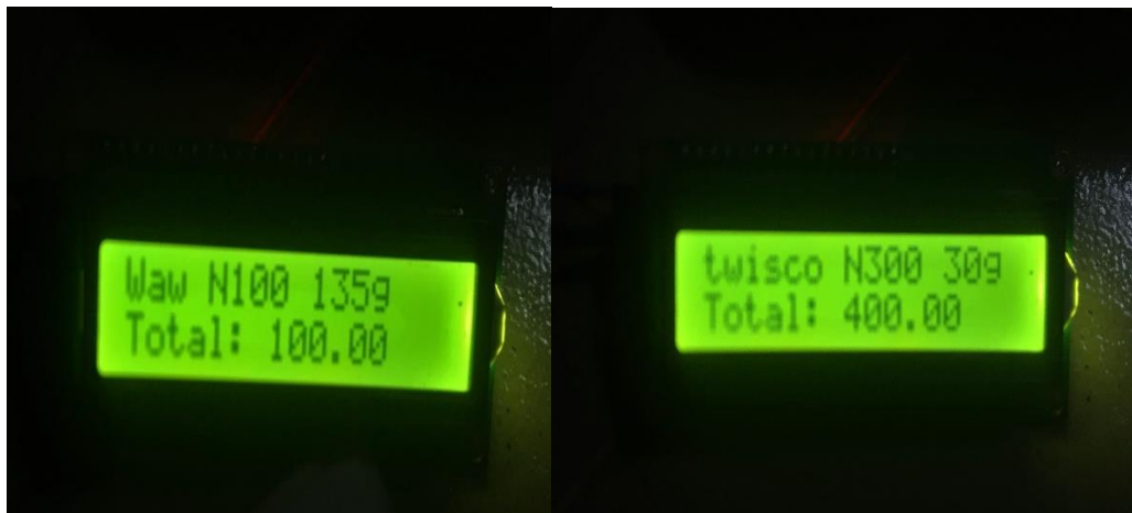
Fig. 6 Showing data read by the barcode scanner displayed on the LCD
