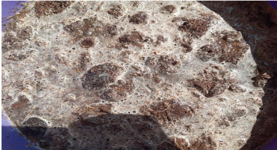
Fig. 3 Substrate (Mixture of cow dung, elephant grass and water)
