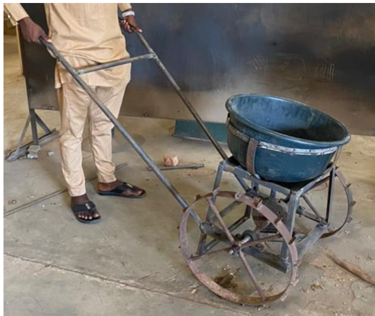
Fig. 1 The Developed Hand-Pushed Fertilizer Applicator
