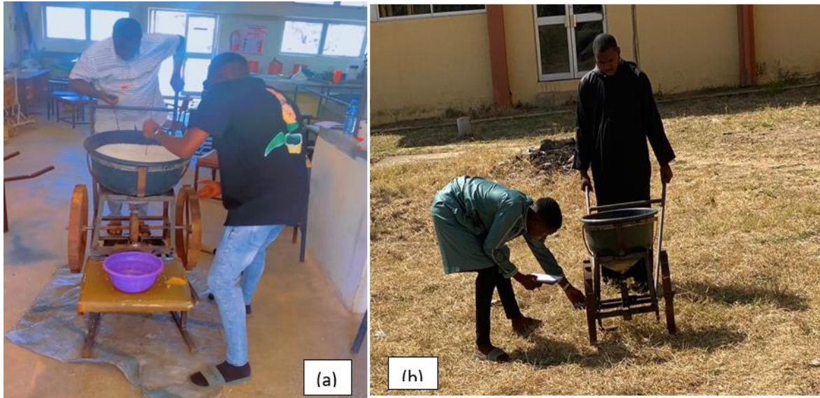
Fig. 2 (a) Laboratory and (b) Field Evaluation of the Hand-Pushed Fertilizer Applicator
