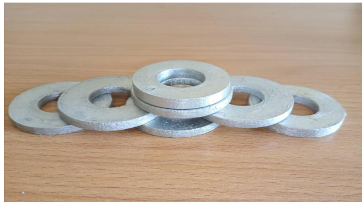
Plate 1. Cast Aluminum Billet with Rings
