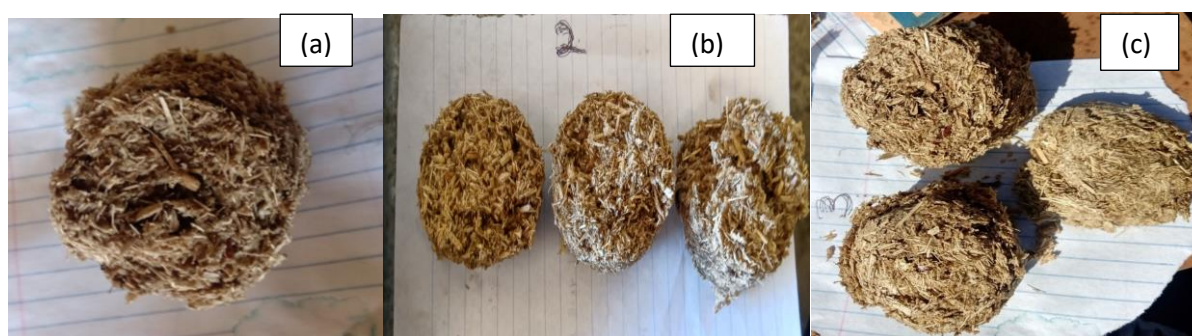
Fig. 2 Briquettes produced from sugarcane bagasse with (a) 7:3 (b) 7:4 and (c) 7:2.5 binder ratios
