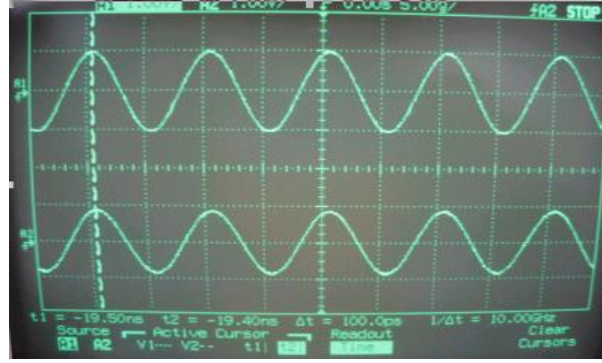
Fig. 7 Output Waveform of Delay Line Displayed on Oscilloscope
