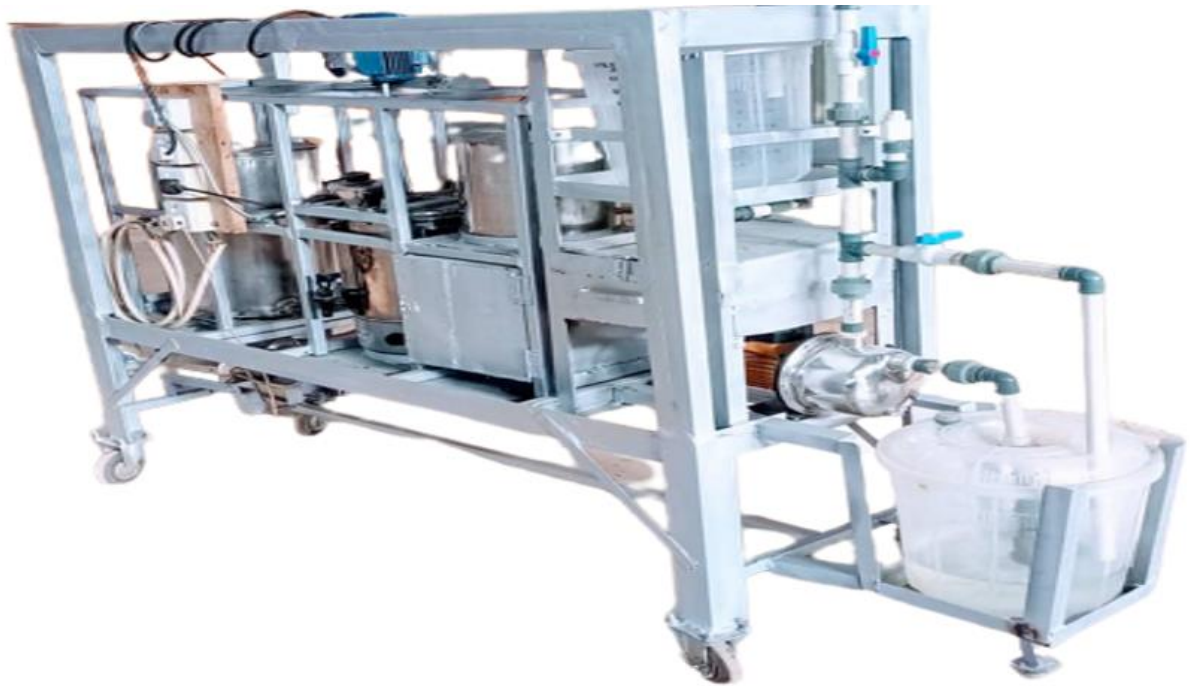
Plate-2 Image of the modified developed Sobo drink plant
