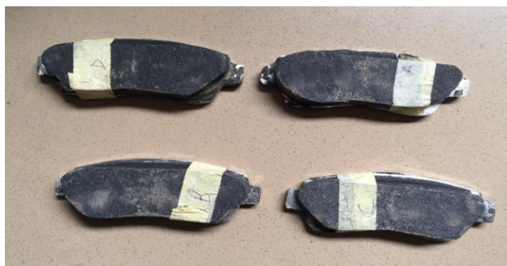
Plate-5 The produced brake pads from biological materials
