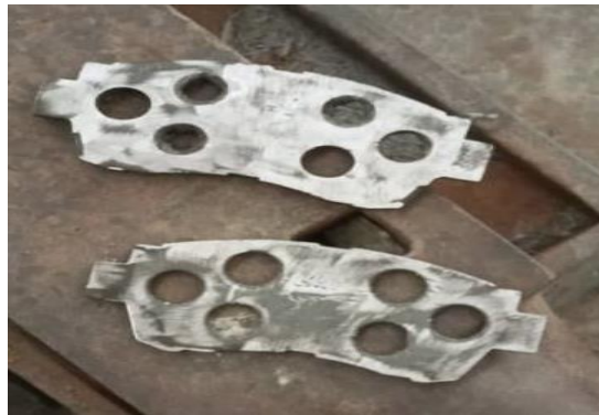
Plate-4 Moulded base material for the brakepad
