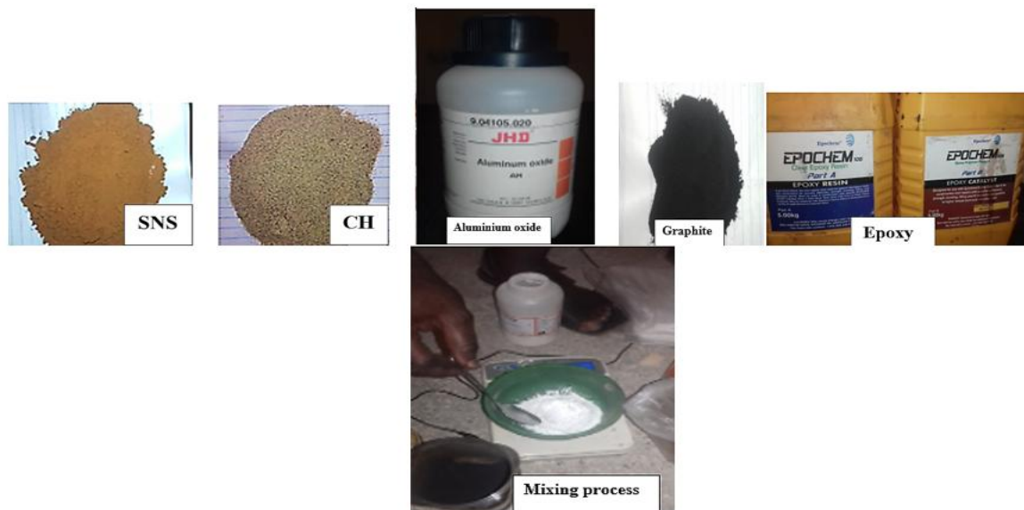
Fig. 2 Materials for brake pad production: a. Epoxy Resin + Epoxy Catalyst, b. Calcium Carbonate Powder, c. Aluminium Oxide Powder, e. Graphite Rods, f. Graphite Powder
