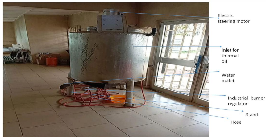
Fig. 1 Three-burner configuration of a double-jacketed mild steel pasteurizer
