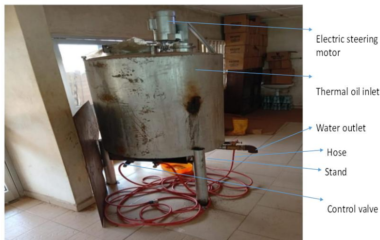
Fig. 2 Four burner configuration of a double-jacketed mild steel pasteurizer
